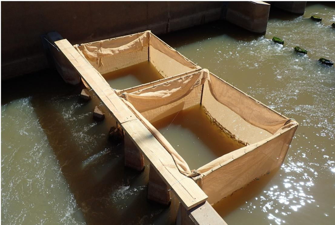
**Figure 9. Cone fishway traps located first resting pool of the fishway during a bottom sample.**
