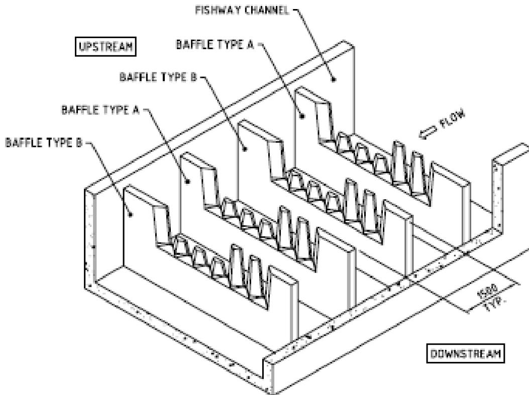
Figure 6. Illustration of the layout of pre-cast cone baffles within the fishway channel.
